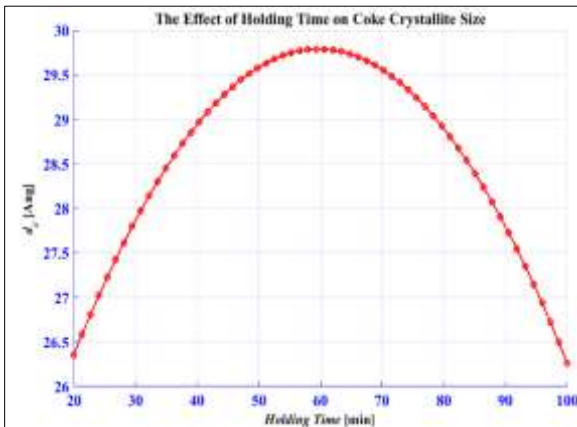
Figure 17. Effect of retention time on crystal size
