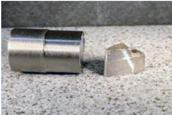
Figure 9. A test sample made of a diamond-enhanced WC-Co tool [10]
