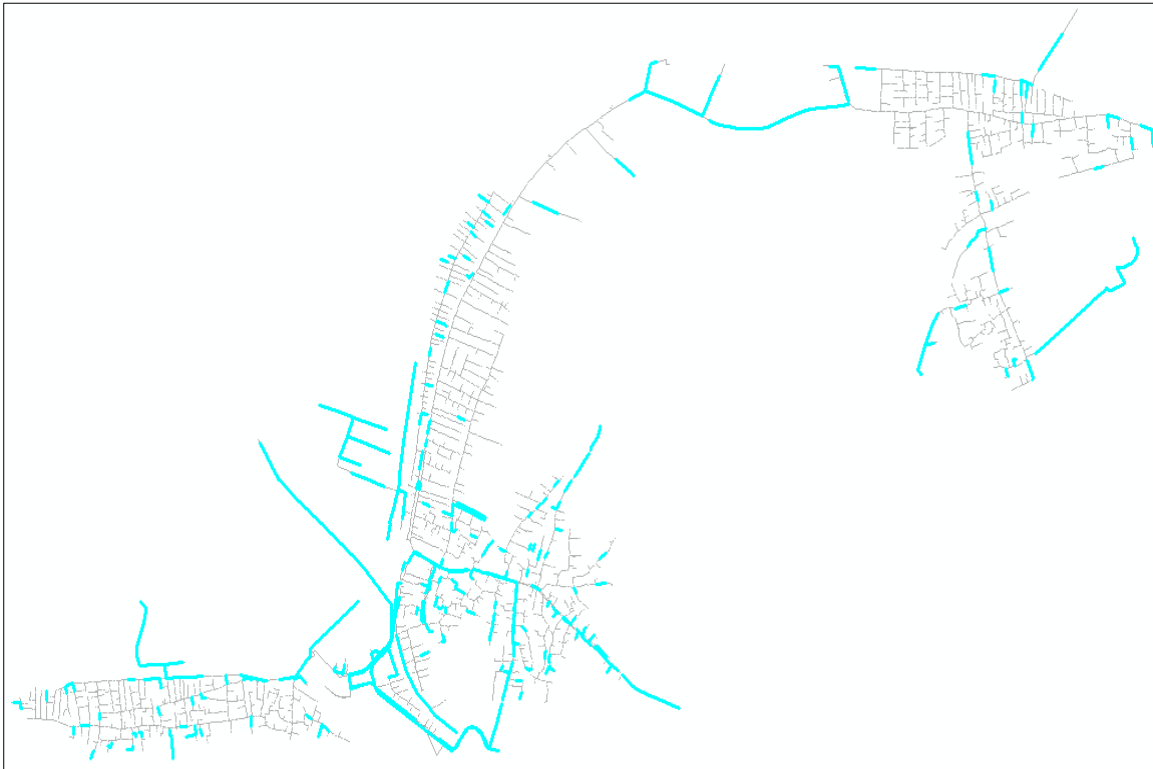
Figure 6. Map of pipes with water leakage risk
