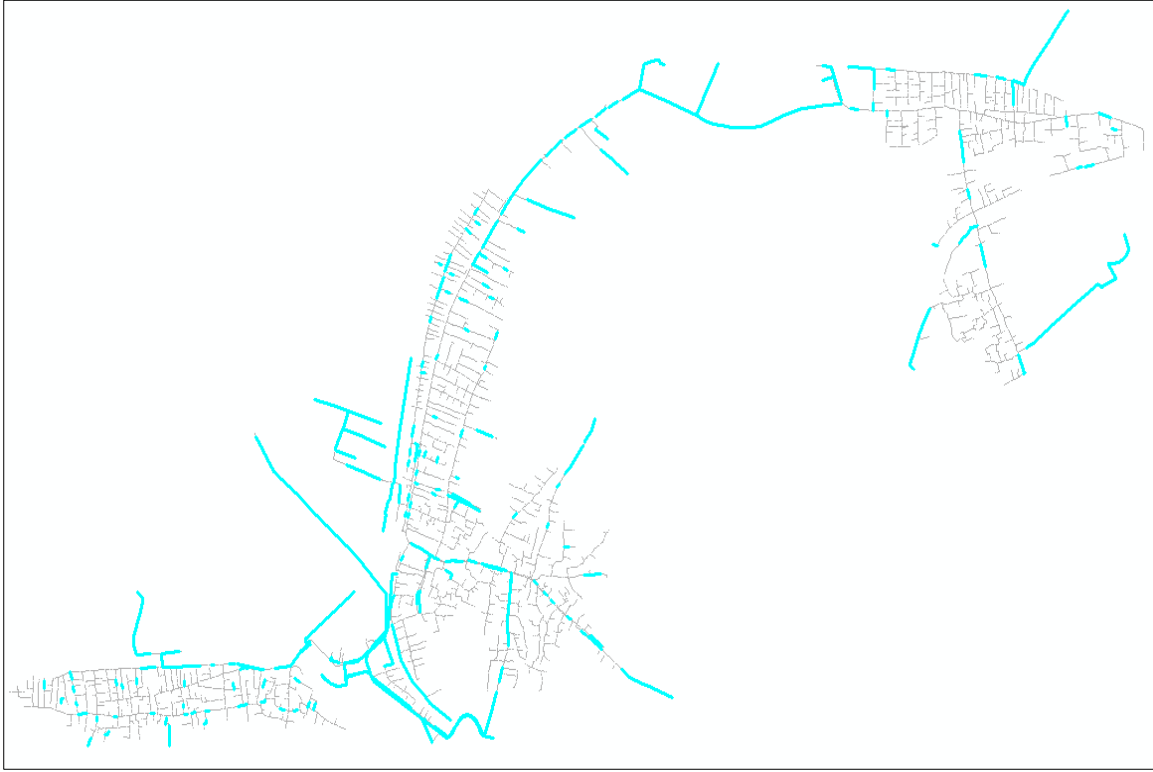
Figure 5. Map of failure risk for pipes
